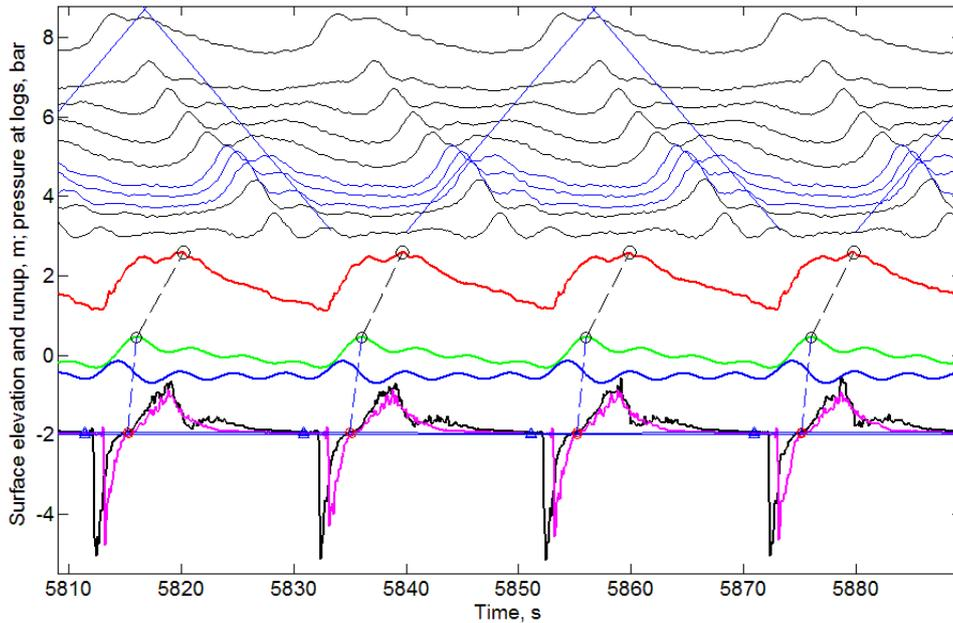
**Fig. 3.** Typical signals. Red: run-up capacitance probe; Thin lines at the top: wave gauges (slope of straight blue diagonal lines corresponds to the wave shallow water phase speed); Green: incident waveform after reconstruction; blue: time derivative of the incident wave; Black at the bottom: force gauge at the log installed at the unperturbed shoreline mark 272 m; Magenta: force gauge at the log installed at 276 m from the wave maker.
