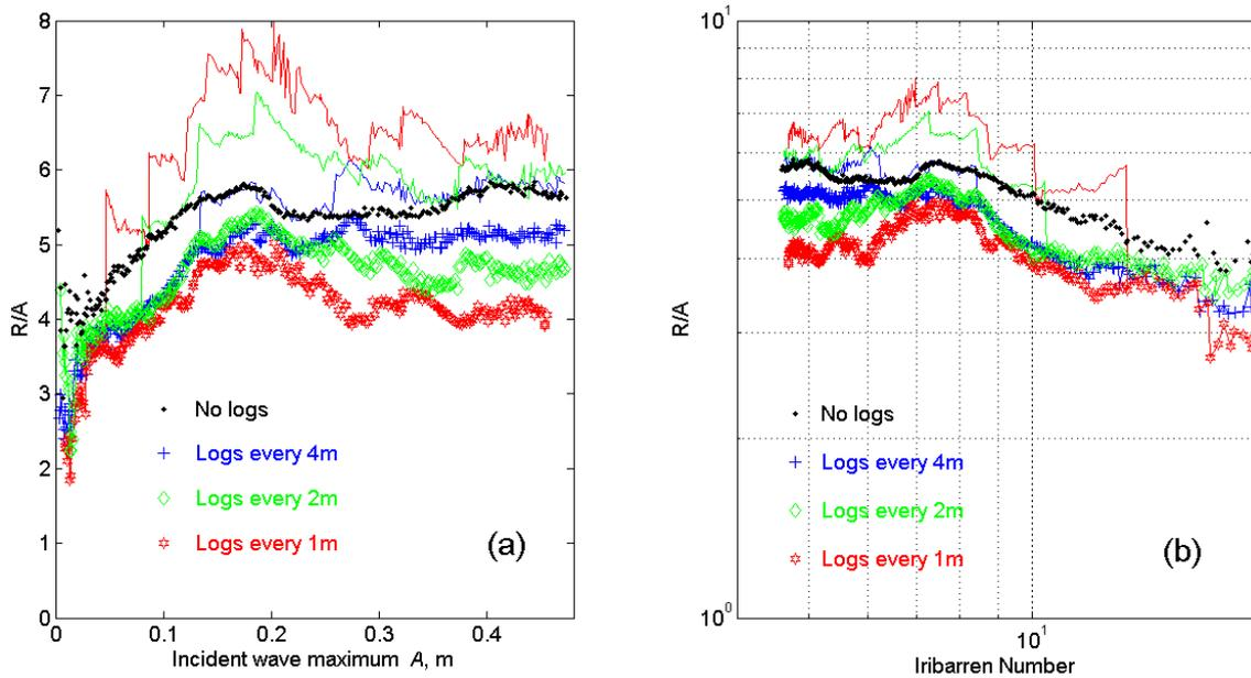
**Fig. 4.** Run-upheight  $R$  vs. incident wave amplitude at different slope roughness. The same data is presented with the maximum incident wave amplitude  $A$  (a) and the Iribarren number (b) on the horizontal axis. Markers correspond to recorded run-up maxima. Solid lines are raised above corresponding marker series by the total sum of heights of the logs the wave encounters on the way up.
