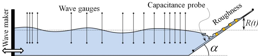
**Fig. 1.** Experimental setup. Large Wave Flume (GWK) with 16 wave gauges, a capacitance probe, and 1:6 slope with “logs” as roughness elements.
