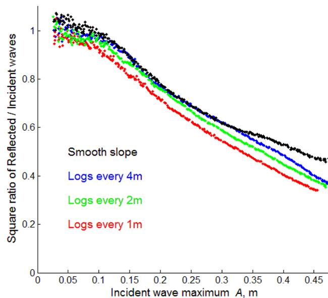
**Fig. 5.** Energy of reflected wave versus wave amplitude at different roughness.
