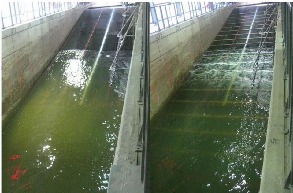
**Fig. 2.** Wave run-up on the smooth plastic slope (left) and on the rough slope with wooden logs installed at every metre. The wave maker is approximately 250 metres behind the camera.
