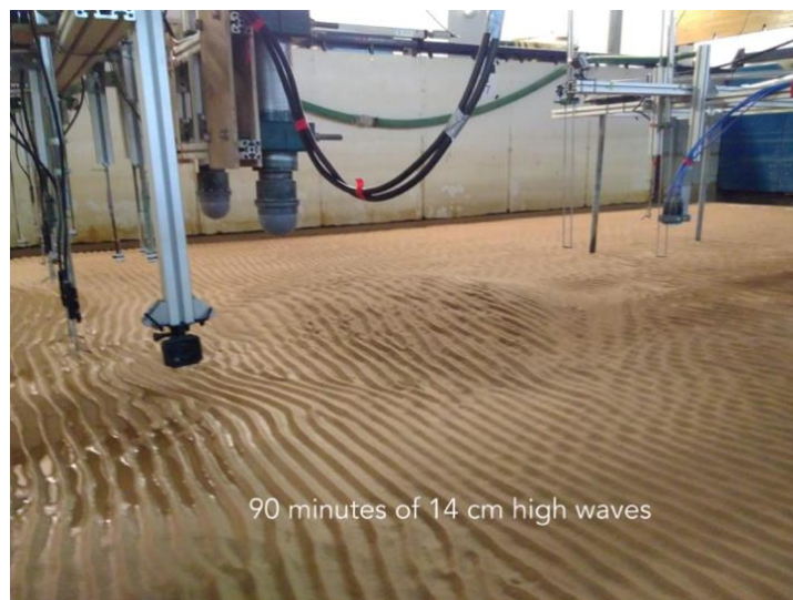
Figure 5 Photo of the bed level after test T2. Paddles of the wavemaker (blue) are visible on the right.
