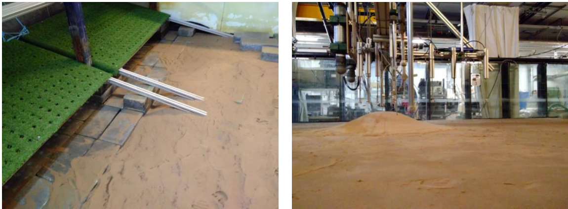
Figure 3 Beach like structure on the downstream side of the flume (left) and the mound prior to a test (right)
