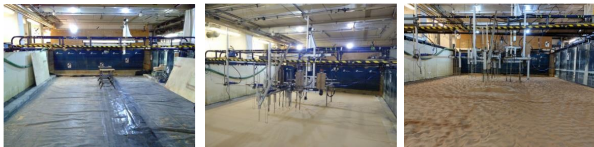
Figure 2 Total Environment Simulator Laboratory setup in Hull, United Kingdom. Photos of the flume prior (left) to the experiment, after filling with sand (middle) and after a test (T4) was run (right). Blue panels on the back wall are the HR Wallingford wave paddles.
