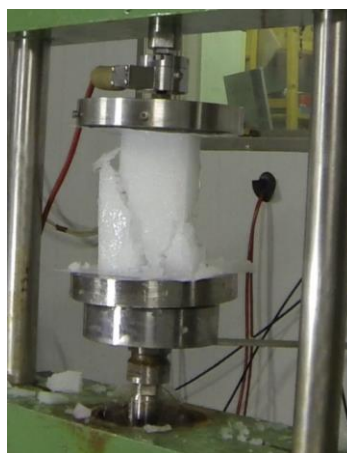
Figure 3. Ex-situ uniaxial compressive strength test.
