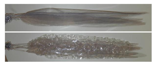
Figure 3.3.2 – Surrogates of L. saccharina as developed by Norvik (2017). Both surrogates are cut with the same shape out of a thin PVC sheet, and undulation on the side of the blades are realized with a heat treatment process. Taken from Norvik (2017).
