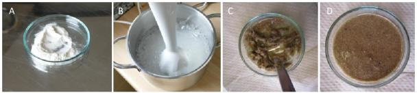
Figure 2.3.5 Mixing procedure. From left to right: A) The surrogate powder is weighted. B) The powder is mixed with water using a stirring blender (~2 mins to destroy larger aggregates). C) The resulting EPS is carefully mixed to sediment (here beach sand) until the dry sediment is completely coated with EPS. D) The surface of the EPS-sediment mix is flattened.
