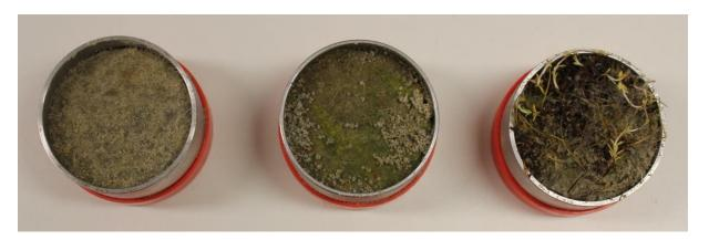
Figure 2.3.2 Sediment cores from Schiermonnikoog. Left: samples without a visible biofilm, Middle: samples with visible biofilm and Right: samples with initial vegetation.
