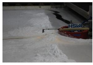
Figure 9: Left: Inclined structure breaking ice sheet by bending upwards. Right: Vertical structure breaking ice by crushing.
