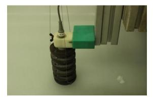
Figure 11: Left: Cylindrical indenter pushed through ice sheet. Right: Strain modulus measured using dead weights over ice sheet and measuring displacement from the middle.
