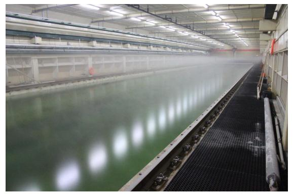
Figure 8: Preparation of model scale ice through seeding in HSVA; the process results in model ice with a columnar structure, similar to the structure of ice in the nature.
