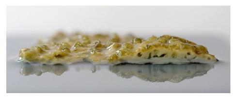
Figure 6: Side-view photograph of biofilm grown on glass beads, University of Stuttgart; maximum thickness of EPS layer is ~5mm
