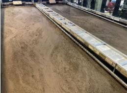
Figure 5: HYDRALAB+ experiments in the Total Environment Simulator, University of Hull: vegetated braided stream during and after flood event
