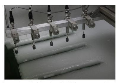
Figure 10: Cantilever beam test: beam is loaded from free-end and displacements measured along beam
