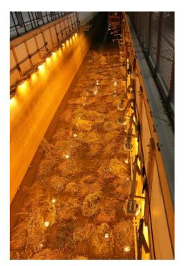
Figure 1: Nature-based solutions: experiments on salt-marsh vegetation in GWK, Hannover
