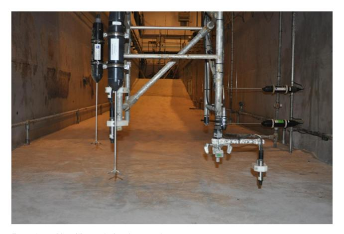
Figure 4: Image of the mobile measuring frame instrumentation.
