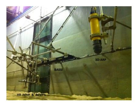
Figure 15. a) Photograph of the instrumentation in the UPC wave flume showing the 3-Dimensional Acoustic Ripple Profiler, 3D-ARP, the Bedform And Suspended Sediment Imager, BASSI and the High Resolution Concentration and Velocity Profilers, HR-ACVP.
