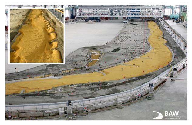
Figure 3 – Illustration of the morphological features developed in the model of the Oder Hohenwutzen conducted at BAW (unpublished work). The model is built with a horizontal length scale of 1:100 and a vertical length scale of 1:40, thus with a distortion of 2.5. Thus, the full length of the model is 80 m, or 8 km in nature. The model bed is made of solid banks with groins and dams and a the movable lightweight sediments are a polystyrene plastic granulate.
